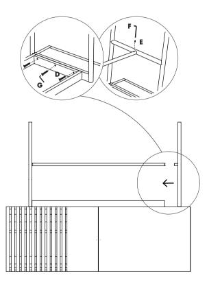
DETACH THE HANDLES FROM THE INSIDE OF THE CABINET AND ATTACH THEM ON THE OUTSIDE OF THE WOODEN DOORS
