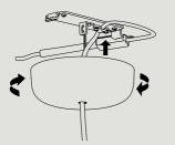
Step 5 Install the plastic canopy onto the metal bracket.
