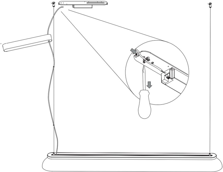
Wiring to mains power: Taking one wire at a time, insert the correct wires into the corresponding slots on the terminal block, while pressing down on the small button next to them. The live mains wire should be inserted into the slot marked L and the neutral mains wire into the slot marked N. If you are unsure of the polarity of the wires, then we recommend you contact a certified electrician.
