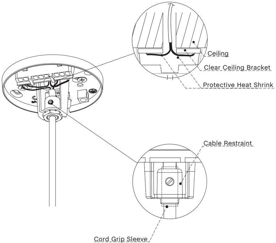
If utilising the mouse hole cable exit, please note the internal cable restraint and integrated cable clamp. The cable clamp tab can be removed and cut to length to suit the cable thickness used, if this is larger than what is already provided. For the source cable, it is advised that any wire exposed with just a single basic layer of insulation is covered with the protective heat shrink provided (Steps 4 – 7).
