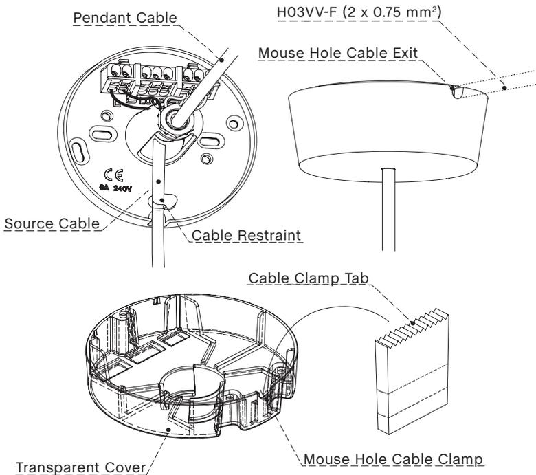
Replace the protective transparent cover over the terminal and clear ceiling bracket, screwing it in place with the three fixings provided. This will isolate the internal electrics during use. Replace the outer magnetic ceiling cap over the assembly, ensuring the mouse hole exits are lined up with the bracket and cap if you intend to utilise this feature.
