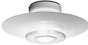
Ceiling fixture providing reflected and diffused lighting. Gloss white powder-coated pressed aluminum reflector. Equipped with special pressed steel support providing a radial starburst pattern. Front shade consists of sand-blasted molded glass and a molded clear glass lens. Matte black painted die-cast aluminum ceiling fitting and gloss white powder-coated pressed aluminum rose.
